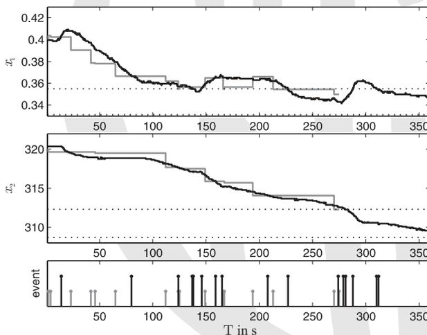
**Figure 9** Trajectories for initial state  $\mathbf{x}(0) = (0.4, 320)$  of the event-based controlled real process (smooth) and simulated process (stairs) using past data on a  $16 \times 16$  grid. The target region is delimited by the dashed lines.
