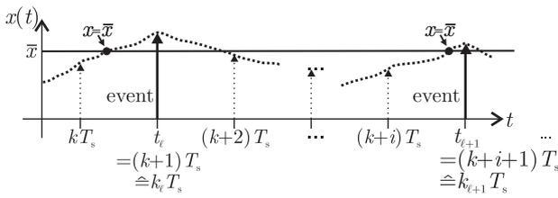
Figure 3 Event-based sampling – discrete-time case.
