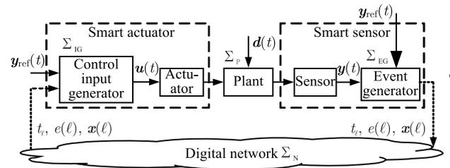
Figure 1 Event-based control loop – continuous-time case.
