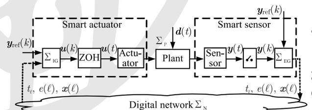
Figure 2 Event-based control loop – discrete-time case.
