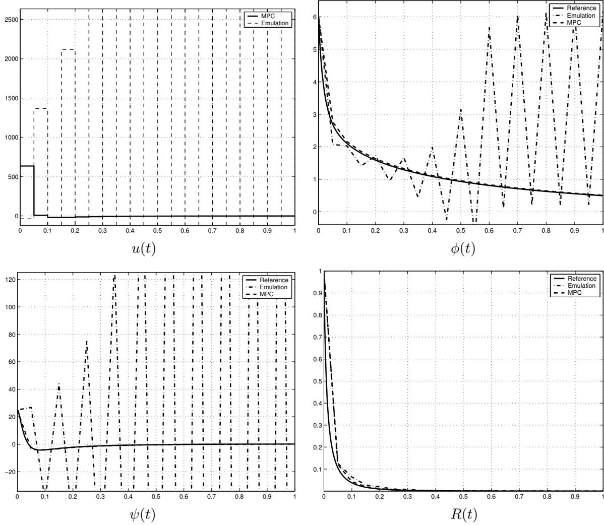
Figure 3.2: Improvement of MPC on unstable emulated controller
